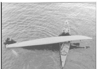
**Step 4:** Slide the over turned boat across the deck until the cockpit is out of the water and water drains out.
